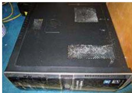
*Just look at the amount of white dust that has collected on the air intake vents of this (tilted-over) mini-tower.*
