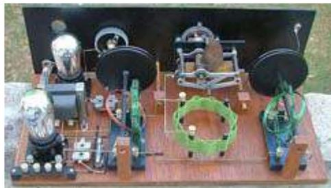
Modern reconstruction by WX4A of a Schnell regenerative receiver design.
