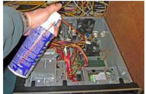
*Using a ‘canned-air’ duster to blow dust and debris away from inside a PC.*
