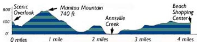
Cross-section of the terrain shows lack of a direct line-of-sight path between the fox's location at the Scenic Overlook and the Beach Shopping Center in Peekskill.
