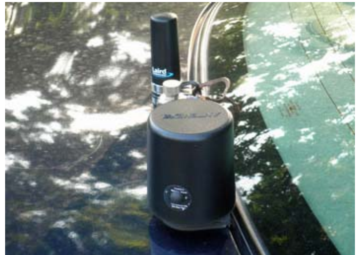
UHF and VHF Laird Phantom antennas mounted on the trunk lip of Marylyn, KC2NKU's vehicle. The VHF antenna looks like an upturned coffee cup. [Photo: W2CH]
