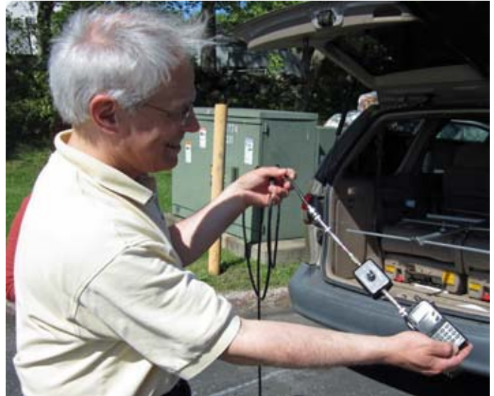
Karl shows his IC-T7H handi-talkie, Radio Shack rotary attenuator, fixed attenuators, all in series with the Yagi antenna stowed in the mini-van.
