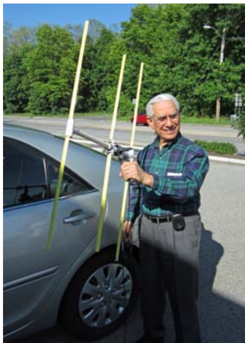
Lovji, N2CKD demonstrates his tape-measure Yagi during the PCARA foxhunt.
