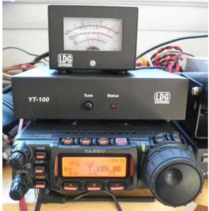
Ray's Yaesu FT-857D multiband transceiver is topped by an LDG YT-100 automatic antenna tuner and an LDG FT-meter. [Photos - W2CH]
