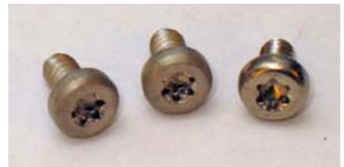
Torx-head screws as used on a disk drive assembly.
