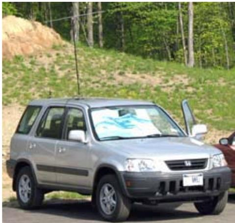
*Fox vehicle NM9J/M, with horizontal dipole mounted on a fiberglass CB whip, radiated 5 watts on 146.565 MHz.*
