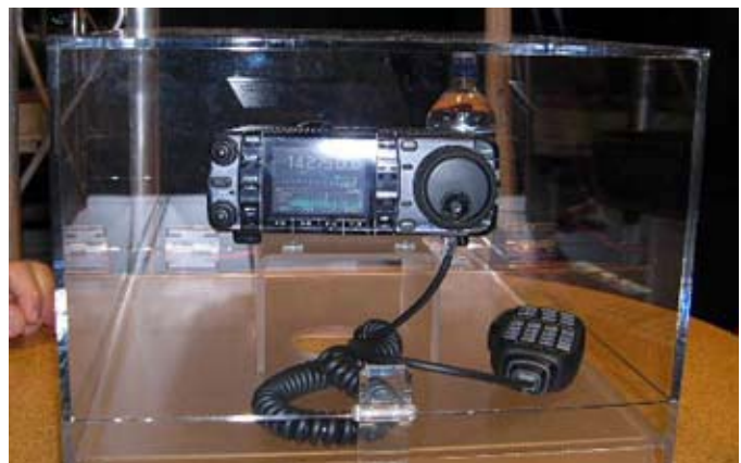
Icom's new IC-7000 transceiver on display. This is an HF-VHF-UHF transceiver, a little smaller than the IC-706MKIIG. It has a multi-color display and puts out 35 watts on 70cm. The front panel is detachable for remote mounting. Ray reports that it should sell for about $1500.00.
