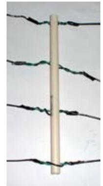
Wire spacers made from plastic pipe
