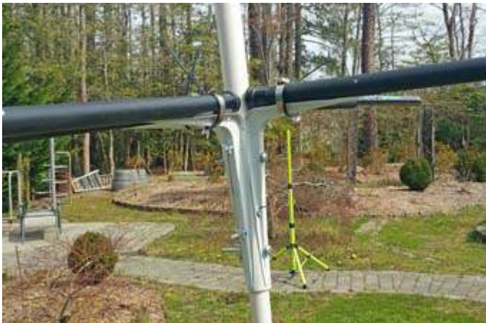
Mount for the fiberglass spreaders in David's Spiderbeam consists of four shelf brackets bolted to a length of 1½" PVC pipe. [K2WPM pics.]
