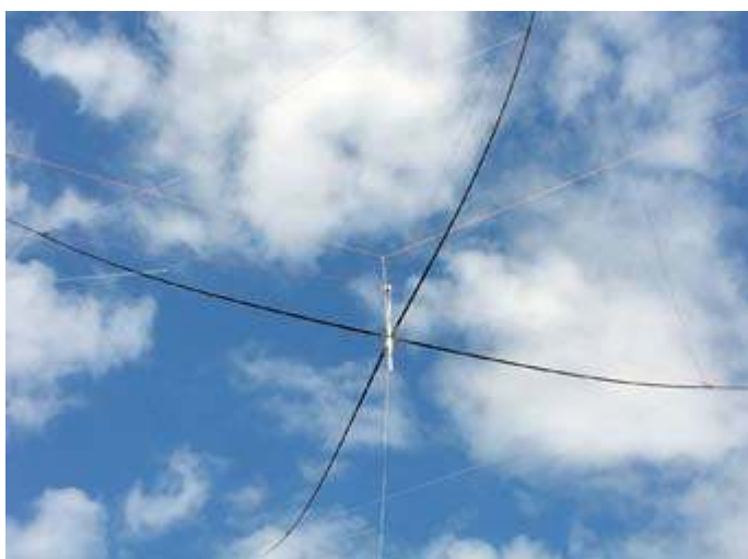
Spiderbeam antenna suspended in the air between two tall trees. The thin wire elements were visible in David's original picture, but only the spreaders and supporting lines can be seen at this resolution. White line at left is an aircraft trail.
