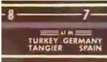
Close up of Grundig short wave tuning dial shows the 41 meter broadcast band (7.1 - 7.35 MHz in Europe).
