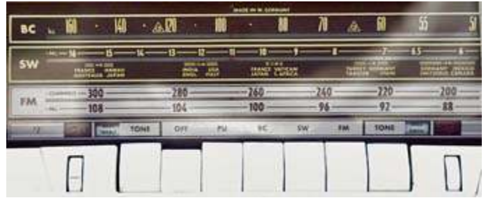
Grundig Majestic piano-key controls and tuning dial.
