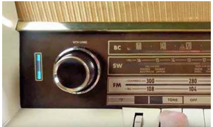
Tuning indicator left of the volume control indicates signal strength. Tone control is also visible lower right.
