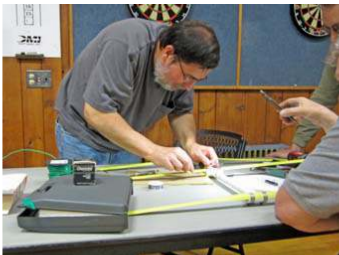
Mike W2IGG prepares to solder coaxial cable to his tape-measure antenna, with illumination from K2WPM's smartphone.
