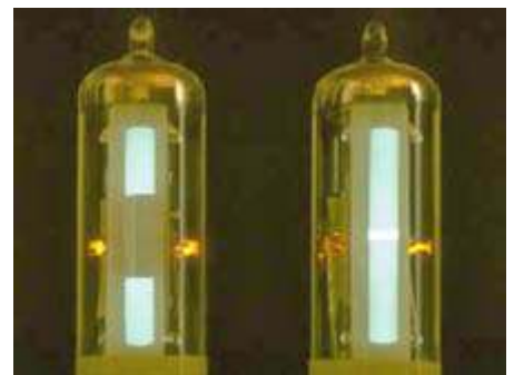
Philips EM87 tuning indicator included a triode amplifier for the AGC line with output controlling electron flow to a bar-shaped fluorescent target electrode.
