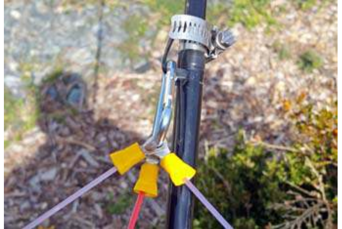
Each fiberglass spreader is supported from the central hub by a length of red weed-wacker line. The ends of the four spreaders are kept in a square configuration by purple weed-wacker lines. Electrical ring connectors are used at the ends.
