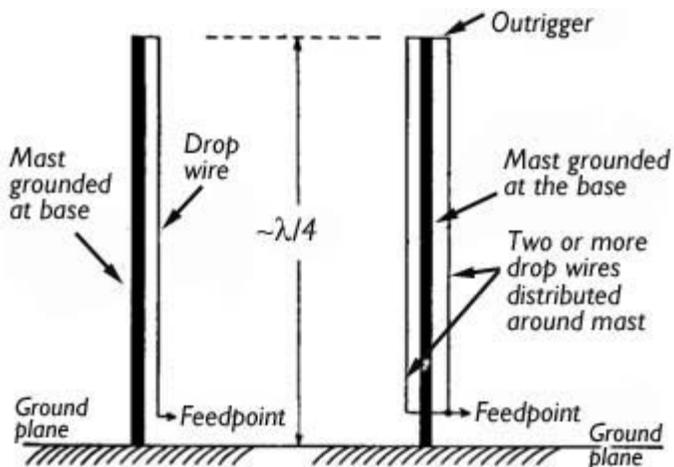
On the left, a folded monopole antenna as used on Radio Caroline. On MV Caroline, a wire cage ran up to the top of the grounded steel mast. On the right is a folded unipole, where a “skirt” consisting of several wires is arranged around a central mast which is also grounded at the base.
