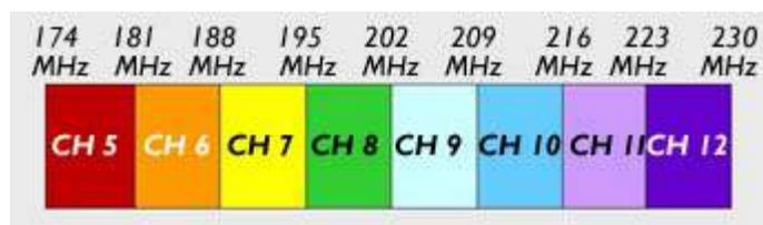
High-VHF Band III TV channels in Europe are now being used for digital radio.
