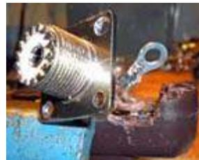
Flexible wires connect the outlet's contact strips to SO-239 center pin and to a solder lug for ground.
