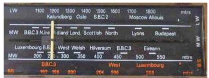
1960s UK transistor radio with “bandspread” (BS) tuning range covering roughly 214-188 meters, 1400-1600 kHz.
