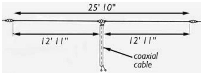
Dimensions of a half-wave dipole for the 17 meter band, center frequency 18.11 MHz, using formula:  $l = 468/f$  ft.
