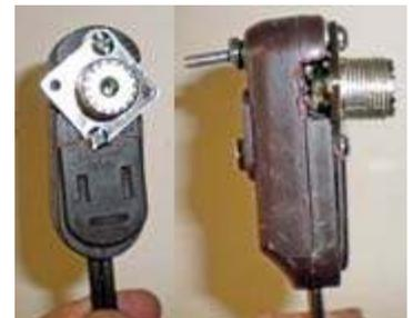
Mount the SO-239 on the molded outlet using machine screws and nuts. [Pics - N2CKD]
