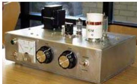
N2HTT's **HF Two Tube** transmitter in final form.
