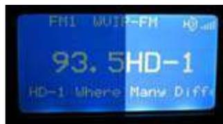
*Effect of tint film (left) on the brightly-lit display of the radio tuner.*
