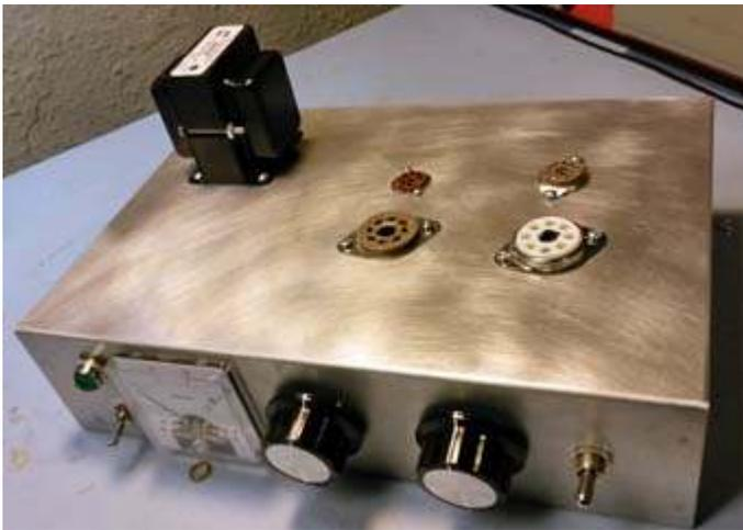
*Aluminum chassis with holes drilled and hardware mounted, prior to component wiring.*
