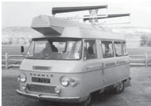
UK Television Detector van, vintage 1968. The roof-mounted antennas were designed to pick up local oscillator radiation from a TV's UHF tuner.
