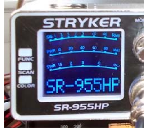
Close up of the LCD display with S-meter, Power and SWR meters plus dot matrix display for readout of settings.
