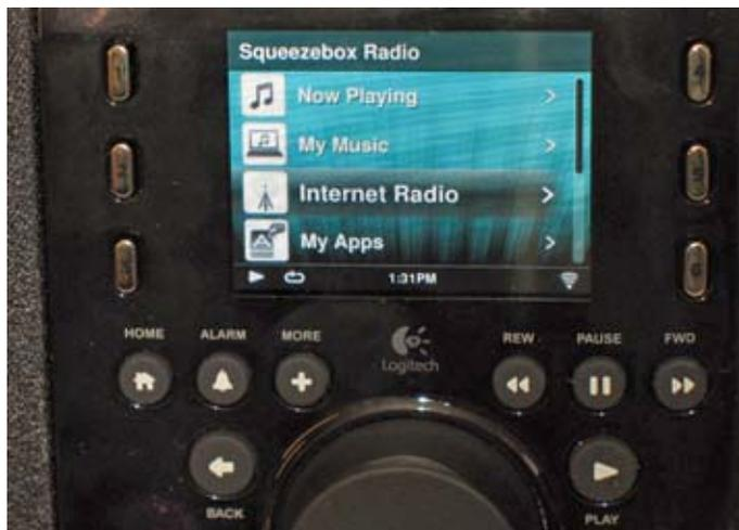
*Closeup view of the Squeezebox Radio showing the LCD color display and front-panel controls.*
