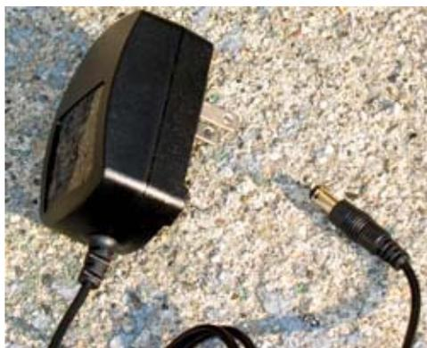
*Logitech switched mode power supply for the Squeezebox Radio is a potent source of interference for any genuine, AM radios nearby.*
