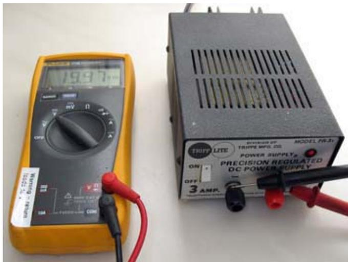
The first thing to check with any second-hand power supply is the output voltage. This TrippLite PR-3a “12 volt” supply was measured at 19.9 volts.
