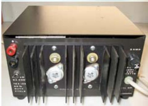
Front and rear views of an Astron RS-12S power supply with built-in speaker. Note the exposed pass transistors on the back.
