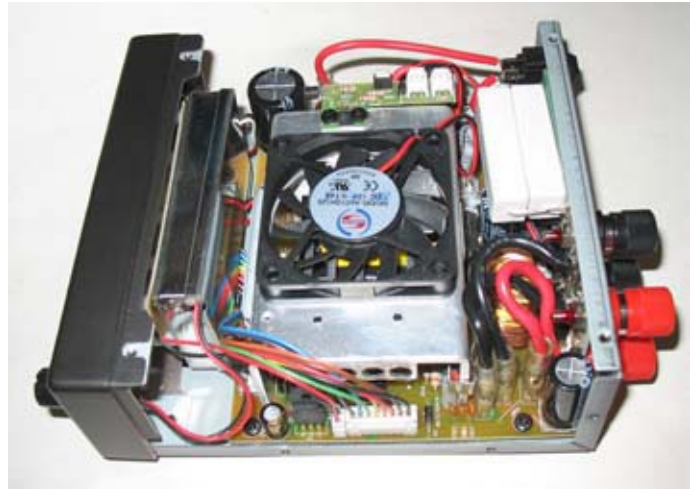
Internal view of Jetstream JTPS14BCM power supply with top cover removed. Note the fan and large heat sink.
