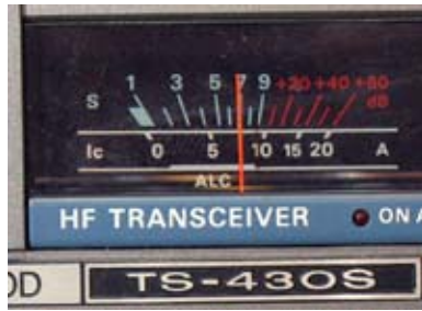
TS-430 S-meter shows noise level on 14 MHz generated by the JTPS14BCM PSU running nearby.
