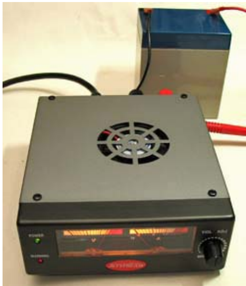
Jetstream JTPS14BCM switch mode power supply. External backup battery is also pictured.
