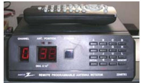
Zenith ZEN-RTR1 rotator console displays location and relative position. Photos by W2CH.
