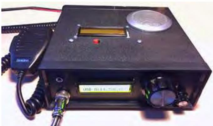
*Todd's μBITX transceiver powered up ready for use. Front panel display reads: USB A:14.300.050. [N2MUZ pic.]*
