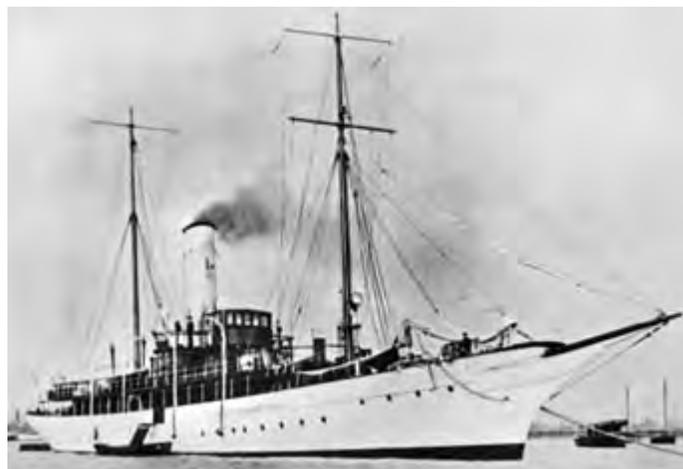
Marconi's 220 ft steam yacht *Elettra* was equipped as a floating wireless laboratory.
