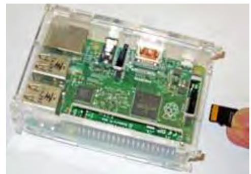
Insert microSD card into the Raspberry Pi card slot **with power off**.
