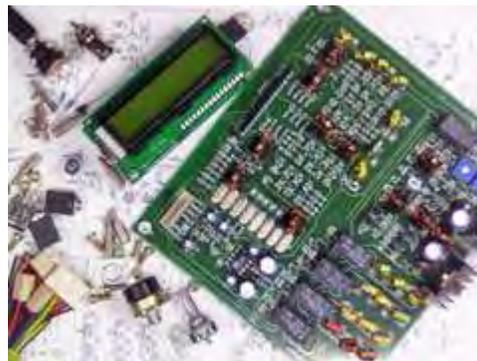
Components in the μBITX kit include a fully tested transceiver board, Raduino board with display, tuning encoder, I/O sockets, BNC connector, electret mic with PTT push button, volume-on/off control, cables and hardware. [HF Signals pic.]
