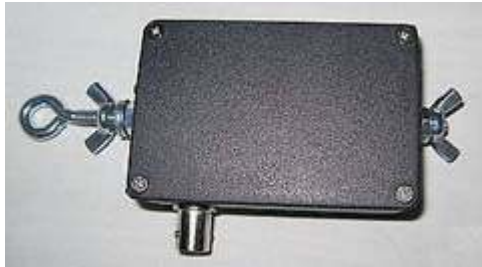
Matchbox for a portable end fed dipole antenna (80-10 meters) is available from “nelson_antennas” on eBay.
