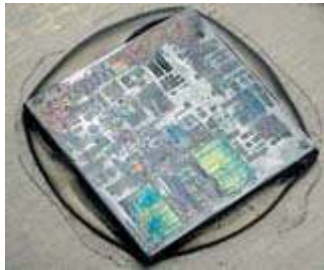
Intel microprocessor chip. How soon will electronic manufacturers abandon silicon for graphene?
