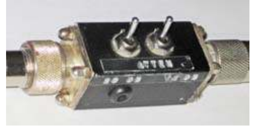
Home-brew passive attenuator with 12dB and 20dB steps for use in foxhunts.
