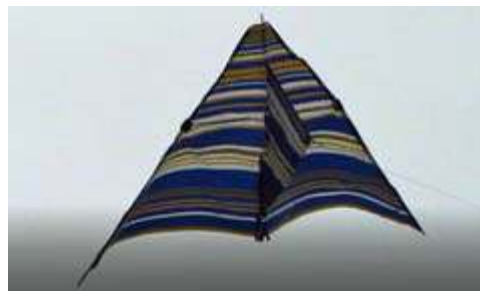
Homebrew 'Delta' kite, photographed in flight. [K2WPM pic.]
