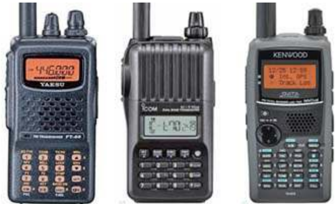
Three recommended dual-band FM handi-talkies. L to R, Yaesu FT-60R, Icom IC-T70A and Kenwood TH-D72A.
