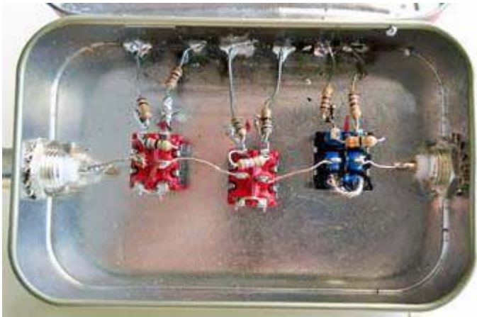
Photo of attenuator shows wiring between the three switches and the two BNC sockets, mounted on the shorter sides of an Altoids tin. [N2CKD pic.]
