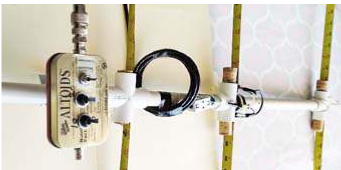
3-step attenuator is mounted to the boom of a 3-element tape-measure Yagi, ready for a foxhunt. [N2CKD pic.]
