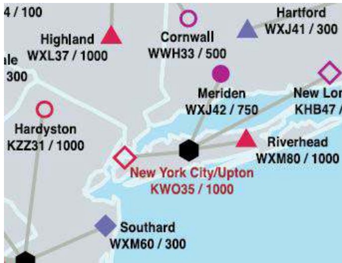
Part of NOAA's map of U.S. Weather Radio transmitter sites, downloadable from http://www.nws.noaa.gov/nwr/ . Symbol shape indicates frequency, symbol color indicates power output.
