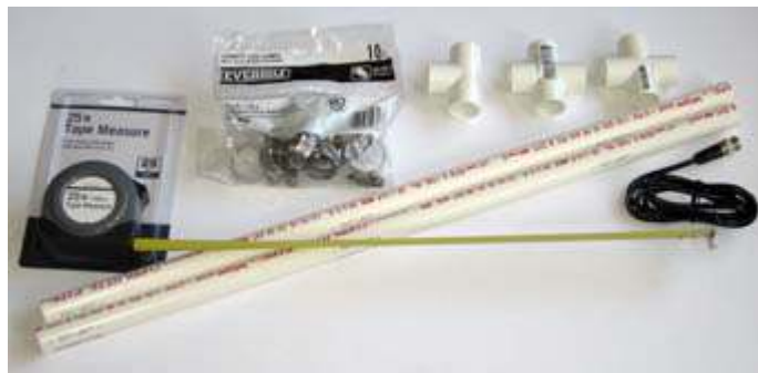
Most of the components for constructing a tape-measure Yagi antenna can be found at Home Depot. (One exception is the antenna cable.)
