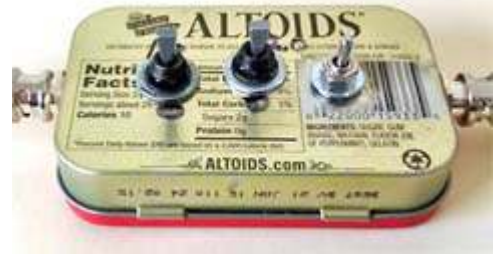
Outer view of the 3-step attenuator showing the DPDT switches [N2CKD pic.]
