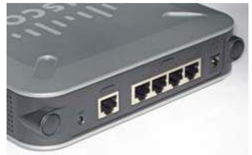
Network router with shielded RJ45 ports for Internet (left) and for LAN.
