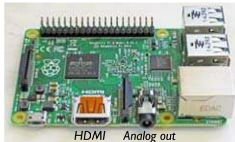
*Credit-card-size Raspberry Pi 2 Model B has an HDMI socket for digital video/audio output and an analog audio jack.*
