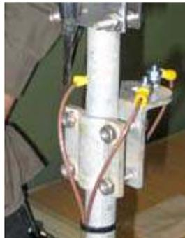
*L-bracket mounted below feed point for attachment of radials.*
