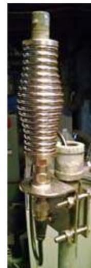
Spring mount with coaxial cable fed through pipe.
