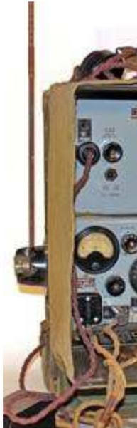
Vertical steel tube antenna attached to side of Wireless Set No. 68.
