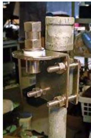
SO-239-to-stud mount attached to sprinkler stand. [N2CBH pic.]
