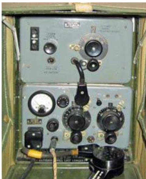
Wireless Set No. 68 was a man-portable transmitter/receiver housed in a steel backpack with canvas cover. RF output was ¼ watt on 1.75 - 2.9/3.0 - 5.2 MHz.
