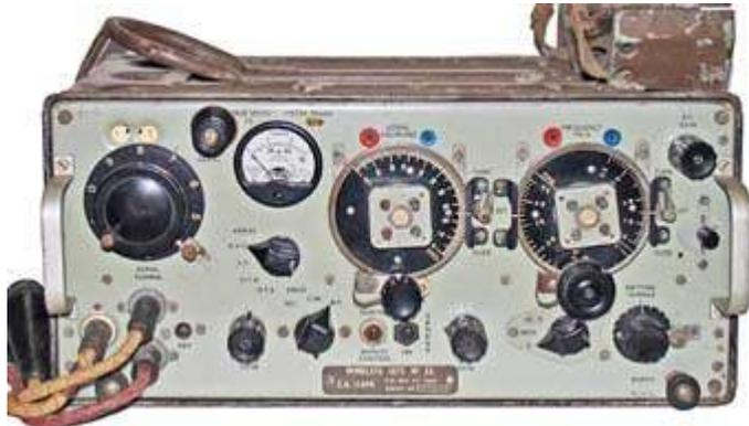
Wireless Set No. 22 was a 13-tube transmitter/receiver for field and mobile use, producing 1 watt RF on 2 - 8 MHz.
