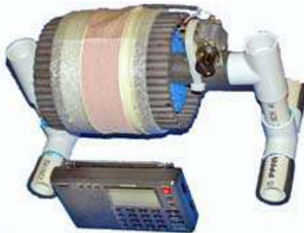
Ferrite sleeve loop antenna built by Gary DeBock is based on 61 ferrite rods.
