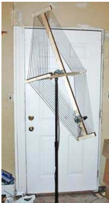
This large box loop antenna built by Bruce Carter can be turned and tilted.
