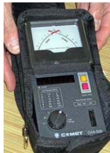
Comet CAA-500 antenna analyzer with its protective cover — as demonstrated by Ray, W2CH.
