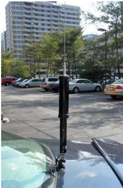
*Diamond SD-330 HF screwdriver antenna mounted on Ray and Marylyn's vehicle.*
