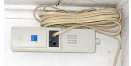
The "thermo-hygro sensor" was mounted high in the breezeway, away from the sun.
