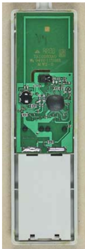
Interior of the TX22U thermo/hygro unit shows the circuit trace (top) for the F-type antenna.
