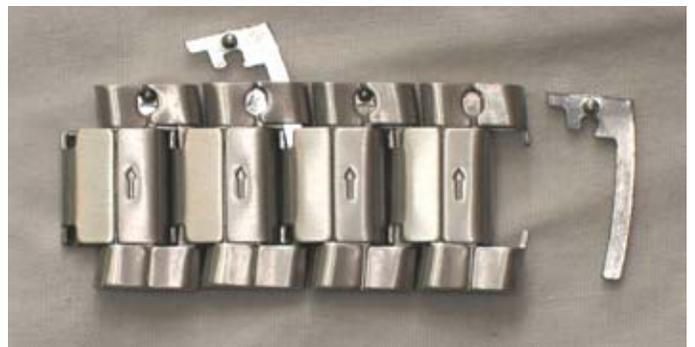
*Removing links from the metal wristband of the Casio WV58DA-1AV.*
