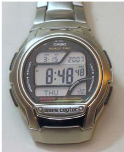
*Casio WV58 watch synchronizes with standard time transmissions on 60 kHz.*
