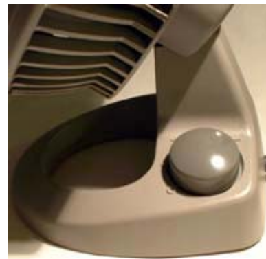
An electric fan with continuously variable speed control can be a terrible source of noise.
