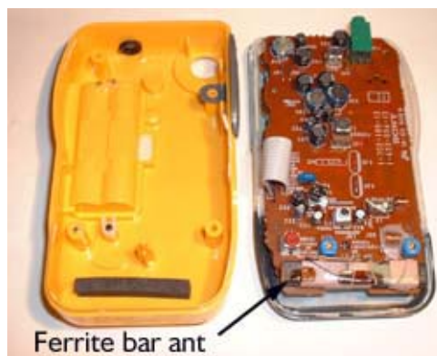
The ferrite bar antenna in a portable AM radio can be helpful in locating sources of interference.
