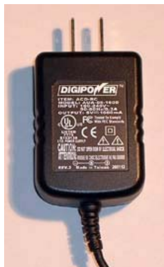
Switched mode power supplies can be a source of interference, especially when antennas are nearby.
