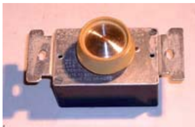
Thyristor-based light dimmers can generate lots of noise at MF and HF. They are best avoided.
