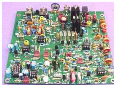
*The OHR-100A circuit board with all components installed.*
