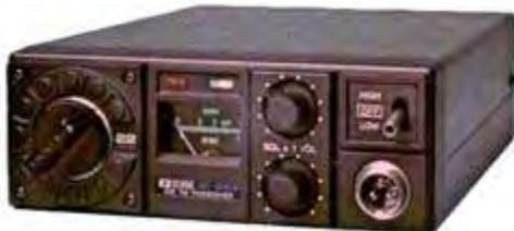
*The Icom IC-22A 2 meter FM mobile transceiver was first imported into the UK by Thanet Electronics in 1976.*
