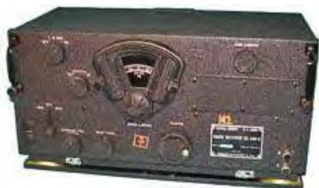
USAAF BC-348 HF communications receiver covered 1.5 - 18 MHz
