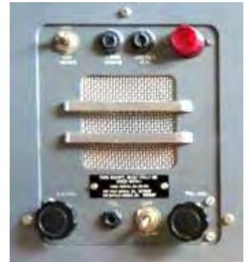
Marconi R220 receiver was part of a 1950s voice system for controlling Anti-Aircraft gun batteries.
