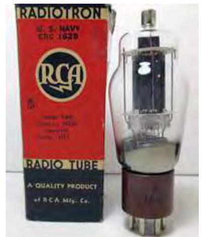
*U.S. Navy 1625 was equivalent to an 807 transmitting tube — with 12.6 volt filament and 7-pin base.*
