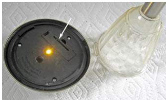
In this solar lamp, the battery cover (arrowed) and LED are visible after twisting the upper body off the plastic bowl.
