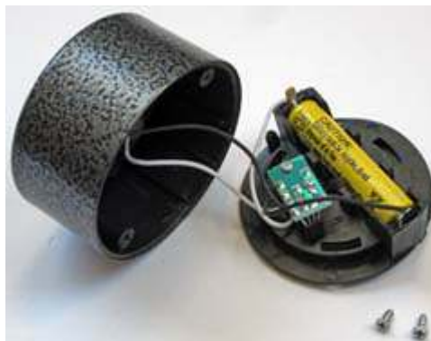
This solar lamp had the plastic body parts secured with two Phillips screws. After separation, AAA-size NiCad cell and controller board are now visible.
