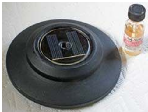
Yard lamp with plastic cover over the solar cell — which had become opaque. The fix was fine sanding and a coat of nail polish.
