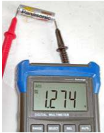
Checking cell voltage with a digital multimeter.
