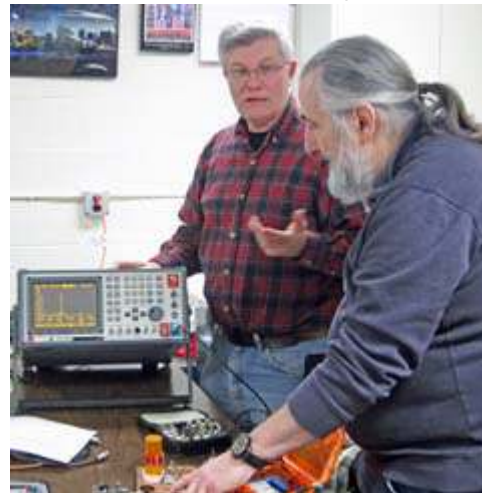
Bob N2CBH checks spectral purity of the QRP TX constructed by Mike N2HTT.
