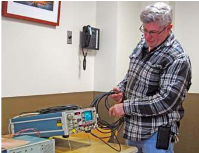
Bob, N2CBH demonstrates use of a Time Domain Reflectometer (TDR) to analyze a length of coaxial cable at the February meeting.
