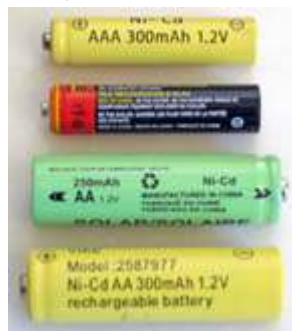
AAA and AA size nickel cadmium cells supplied with solar lights. Capacity 250-300 mAh.
