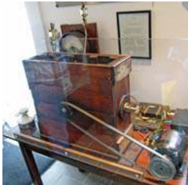
“Old Betsy” rotary spark gap transmitter as used by Hiram P. Maxim around 1920, on display at WIAW, ARRL Headquarters.
