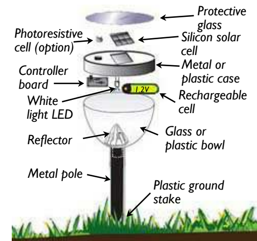
Construction of typical solar yard lamp.
