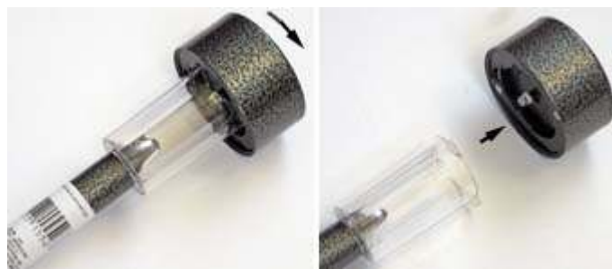
This solar yard lamp was disassembled by twisting the metal body and lifting away from the plastic bowl.
