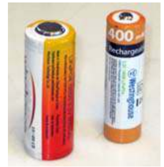
LiFePO 4 cells supplied with higher-power solar lights. Capacity 600 - 400 mAh.
