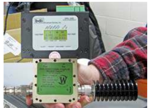
Bob demonstrates the BDI DPS-100D digital RF power measurement system.
