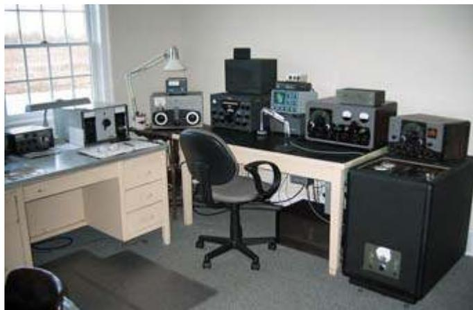
*The K2VXV radio room features (L to R) Drake R4C/T-4XC separates and Henry 2KD-5 linear, EF Johnson Viking KW Matchbox, Collins 75A4 receiver, Heath monitor, Viking 500 transmitter, and Viking Ranger 1 transmitter atop the Viking Desk Kilowatt power amplifier.*
