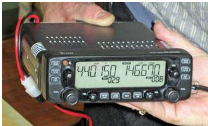
Icom IC-2730H in the hands of Ray, W2CH, is a dual-band mobile FM transceiver covering 2 meters and 440 MHz.
