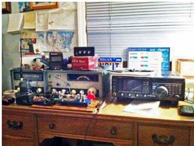
*Karl's current shack features a Heathkit HW-16 CW transceiver with external VFO to the left and recently-acquired Yaesu FT dx 1200 HF transceiver to the right.*
