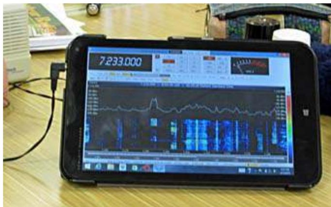
Remote operation of a software defined radio using SDR-Radio.com software, as demonstrated on 40 meters by N2EAB at the February meeting.
