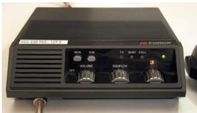
Uniden AMU 250 after conversion to 440 MHz, with new panel lamp in place.
