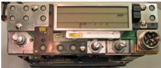
IC-3200A with plastic front panel removed.
