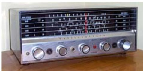
*Hallicrafters S-120 receiver covered 540 kHz to 31 MHz on AM and CW.*
