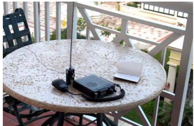
Ray's portable station consists of a Yaesu FT-817ND QRP transceiver and Miracle Whip antenna.
