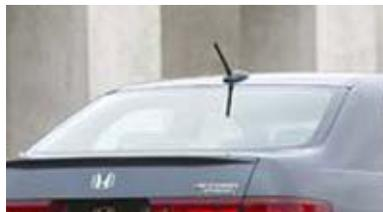
2005 Honda Accord Hybrid has a combined AM/FM/XM antenna.
