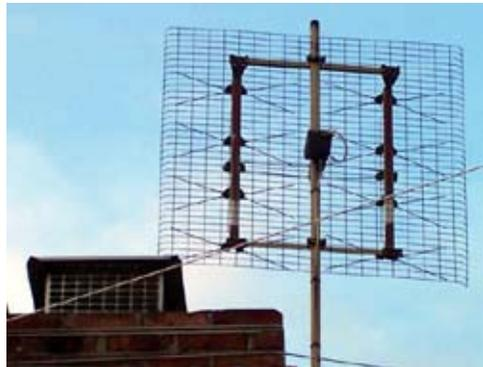
*Channel Master CM4228A 8 bay bow tie UHF array used by N2KZ for digital TV reception with a LG 3100T set top box.*
