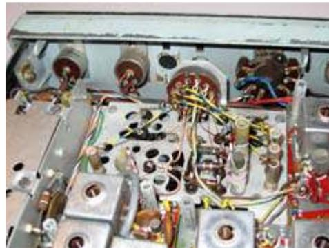
*View below chassis shows front panel with rotary controls for (L to R): volume, squelch, 6-way channel switch and power switch. Center hole is no longer used.*
