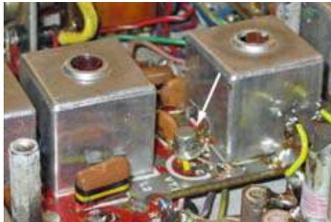
1st RF amplifier transistor VT1 (arrowed) on the R.F. Unit board was changed from an AFZ12 to low-noise UHF type AF239.
