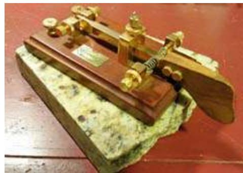
LTA cootie key, mounted on a chunk of granite countertop [N2HTT pic].
