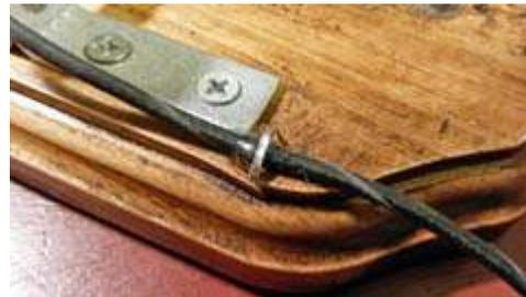
*Cable strain relief consists of a staple and dab of hot-melt glue.*
