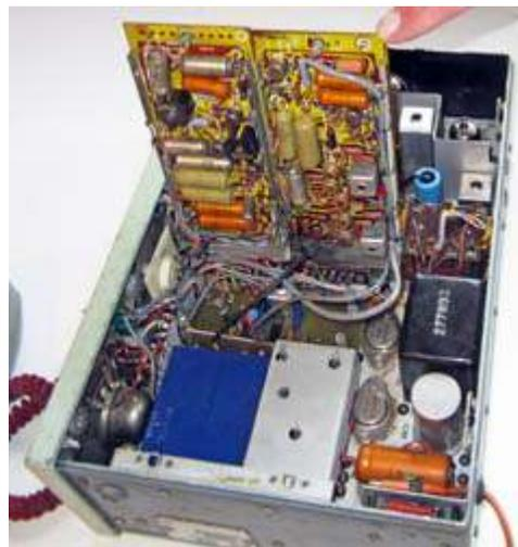
*View above chassis shows the A.F. Section and Second I.F. Unit boards hinged-up, revealing the blue Block Filter, lower left.*
