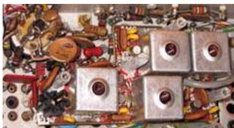
*A.J.H. Electronics phase modulator board installed in the modified Pye Cambridge.*
