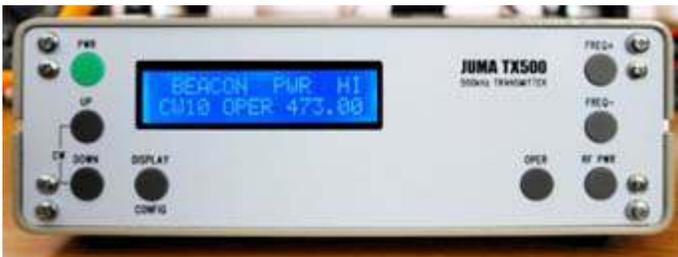
The Juma TX500 is a digitally-controlled 60 watt CW transmitter from Finland intended for the 630 meter band.
