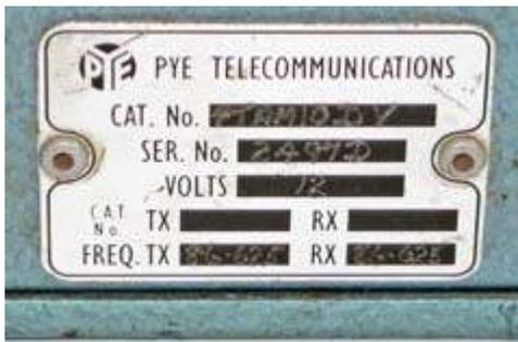
*Serial plate on side of the Pye Cambridge shows catalog number, serial number, voltage and frequency information.*
