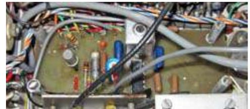
Garex FM detector board mounted in Pye Cambridge in place of the Squelch Unit.
