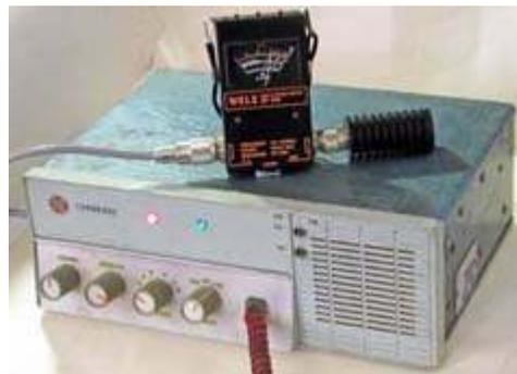
*Testing power output from the 70 MHz Pye Cambridge after 30 years in storage.*
