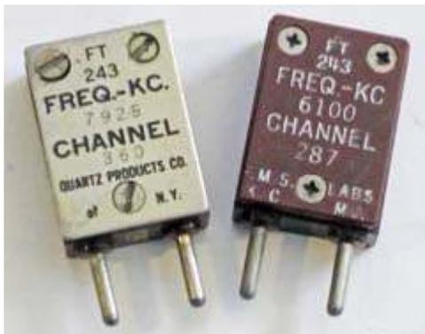
Out-of-band FT-243 crystals from World War II can be ground or etched to a higher frequency — or used to hold a smaller quartz crystal.
