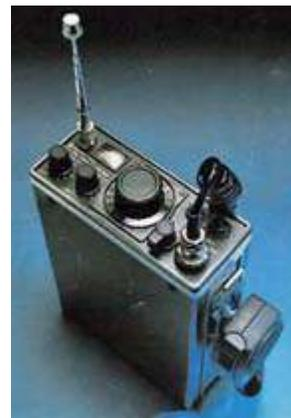
*Trio-Kenwood TR-2300 1 watt portable FM transceiver for 144 MHz.*
