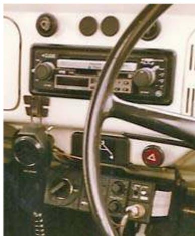
*The Beetle had right-hand drive, a Sharp synthesized cassette-radio and a crystal-controlled Icom IC-22A transceiver for 2 meters.*
