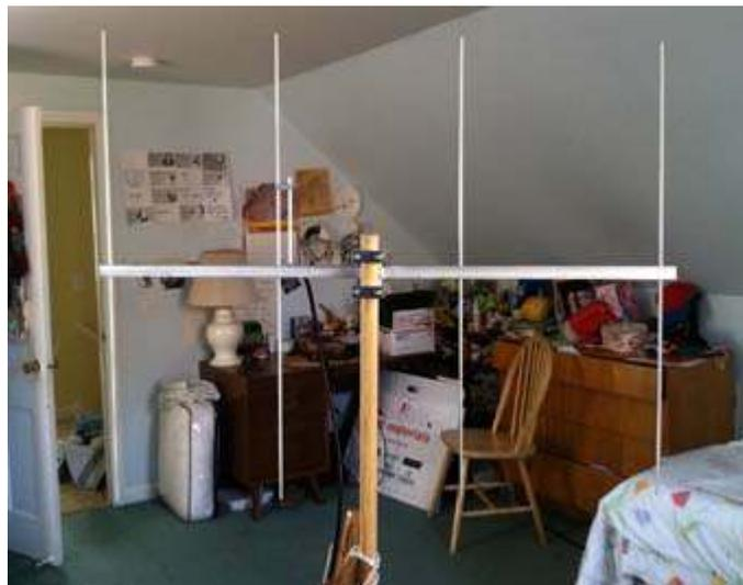
*Arrow 146-4S four-element Yagi for 2 meters.*
