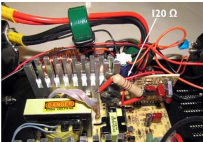
*Addition of 120 ohm resistor across the thermal switch in the SS-30M power supply.*
