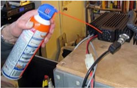
Using "Blow Off" canned air to remove dust from a cooling fan.
