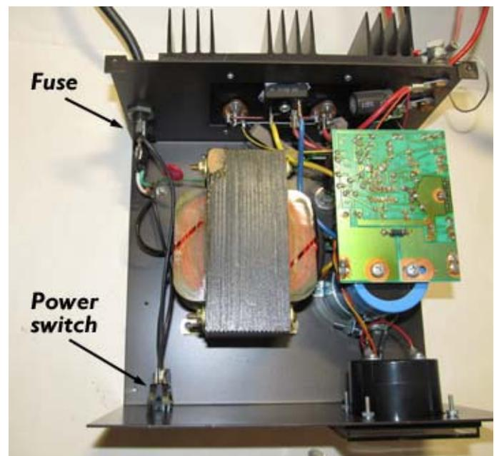
*Astron RS-20M power supply with the cover off. High voltage is exposed around the 120 volt connections for the fuse and the power switch*
