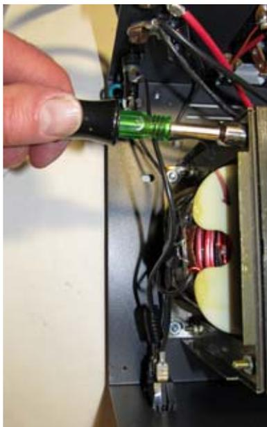
*Using a nutdriver to tighten hardware on the mains transformer within an Astron RS-35A power supply.*
