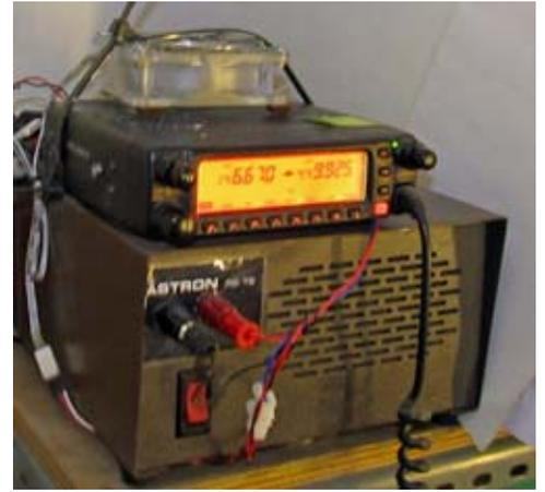
Cooling fan sits on top of Yaesu FT-8000 as part of IRLP node 4214. A second fan is behind the radio, cooling the Astron RS-7S power supply.
