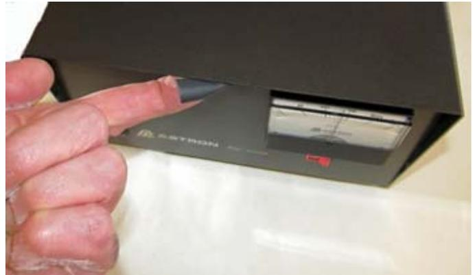
*Preventing vibration by sliding a piece of rubber sleeving into the gap between top cover and front panel on an Astron RS-20M.*
