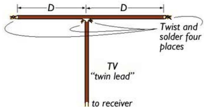
Folded dipole can be assembled from 300 ohm TV twin lead. A balun is needed to match to 50 ohm coaxial cable.
