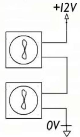
Two 12 volt fans wired in series will run quietly from a 12 volt supply.
