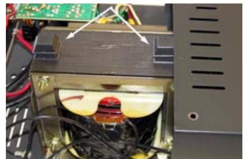
*Rubber cushion feet (arrowed) on top of transformer to prevent steel cover vibrating.*
