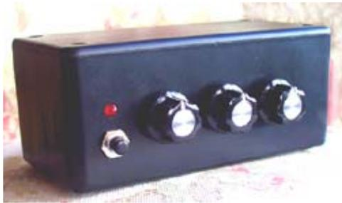
Hi-Mite 20 meter transceiver in case with three knobs.
