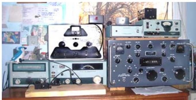
*The N2KZ shack includes (left to right) Heath HG-10B VFO alongside Heath HW-16 CW transceiver; on top is Heath DX-20 CW transmitter. To the right, down on the desk is the Collins-designed R-390 receiver, with Heath HW-7 CW QRP transceiver sitting on top.*
