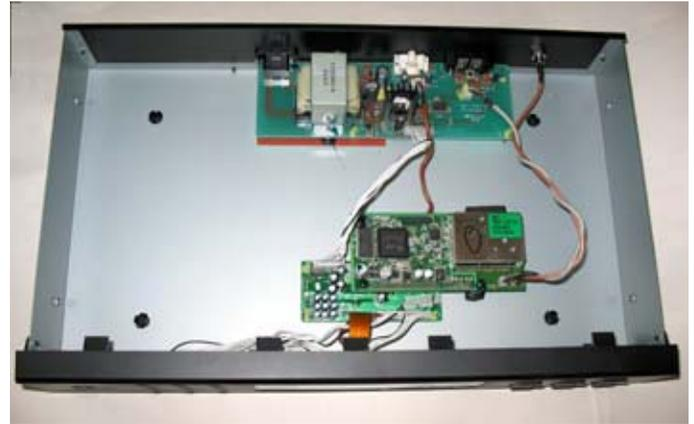
*Sangean HDT-1 metal case is almost empty. RF tuner and DSP stages are on the circuit board near the center.*
