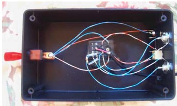
*Transmit-receive switch handles antenna switching and keyer control for Karl's separate transmitter and receiver setup.*
