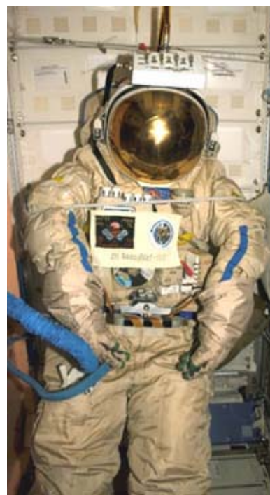
SuitSat-1 ready for launch. The electronics control panel is on top of the helmet along with the SuitSat antenna. [Photo courtesy NASA.]
