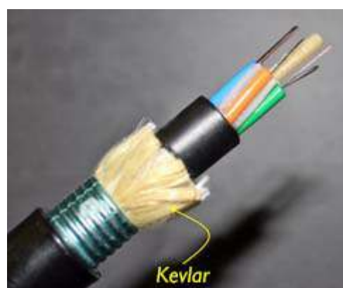
Fiber-optic aerial cable with Kevlar yarn wrapping for protection. [DuPont pic.]
