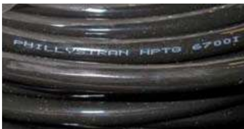
Phillystran HPTG 6700I tower guy line has a breaking strength of 6700 pounds.
