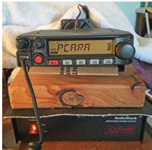
Yaesu FT-1900R transceiver with cooling fan at rear.
