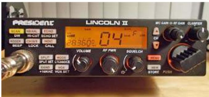
*Lincoln II front panel showing the fourteen push buttons, most of which are dual-function. [W2CH pic.]*
