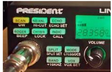
*Close-up of the Lincoln II left front panel showing ten of the push-buttons. Choosing a backlight color of green affects both the display and the backlit buttons [W2CH pic.]*
