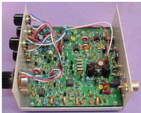
Oak Hills Research OHR-100A CW transceiver kit as constructed by Karl for the 30 meter band.
