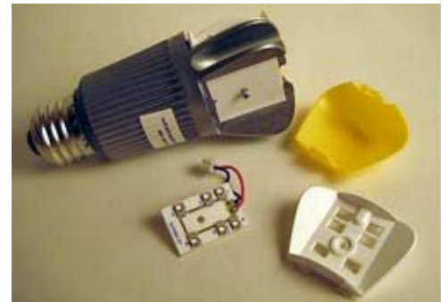
Components of a Philips "remote phosphor" LED lamp.
