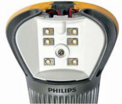
Philips "remote phosphor" design moves the yellow phosphor away from the LEDs to the outside of the lamp.
