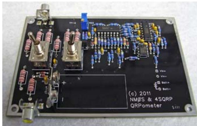
*QRPometer main board showing mounting space for the 9 volt battery.*
