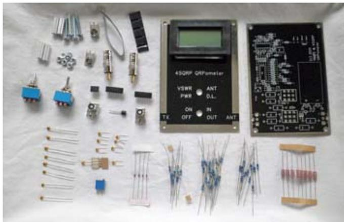
*QRPometer kit with parts laid out ready for construction [Photo - W2CH]*
