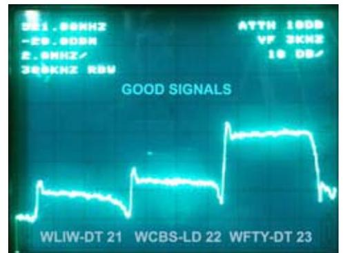
Scan of three adjacent UHF digital TV channels transmitted from Long Island. Left to right, WLIW-DT, Garden City, NY on channel 21; WCBS' digital fill-in translator on channel 22 from Plainview, and WFTY-DT, Telefutera, Smithtown, NY on channel 23. Note the flat spectral response in each case.
