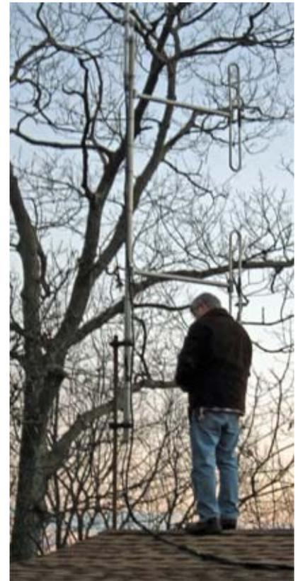
Bob N2CBH checks the Sinclair stacked dipole antenna on Nov 25.
