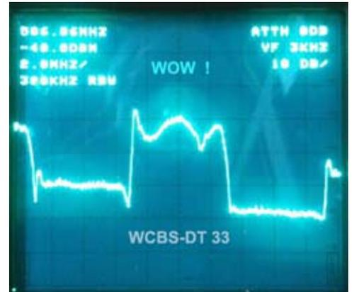
Scan of UHF digital TV transmission from WCBS-DT on channel 33. Screenshot from Tektronix 2710 spectrum analyzer.
