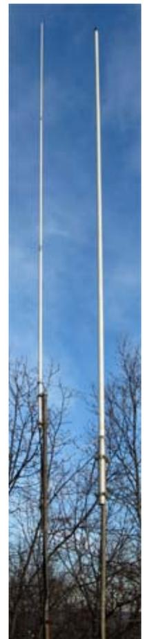
*New arrangement with Diamond X500 for 449.925 on left and Super Stationmaster for 146.67 on right.*
