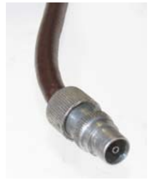
UK 75 ohm low-loss coaxial cable fitted with a Belling-Lee connector.
