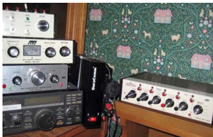
WOERE/B beacon transmitter uses an MFJ-9030 30 meter CW transceiver.
