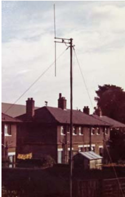
G3VNZ full wave vertical for 2 meters was made from cut-down VHF TV antennas. (That's Southport Football Club in the background.)
