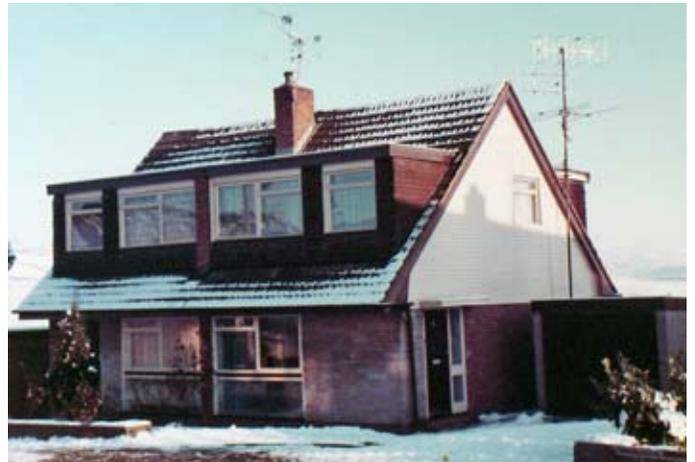
The G3VNQ location on a snowy day in Rochdale, UK. Rotary VHF antennas at right included a 2 meter cubical quad, 430 MHz 8 over 8 and a 3 ele Yagi for 70 MHz.
