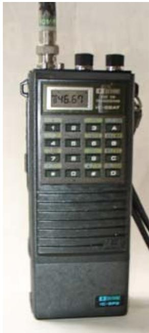
*The first radio I purchased in the USA was this Icom IC-02A 2 meter FM portable.*
