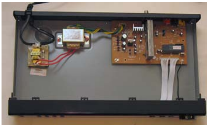
Insignia tuner with top cover removed. Small board on the left is a 120V AC line filter. The main circuitry is all contained on the circuit board at right.
