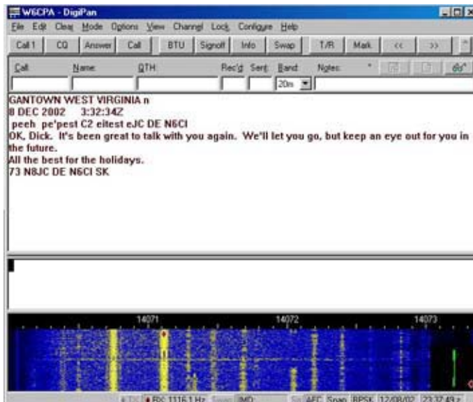
Screen shot of Digipan software, decoding PSK31 transmissions on 20 meters.
