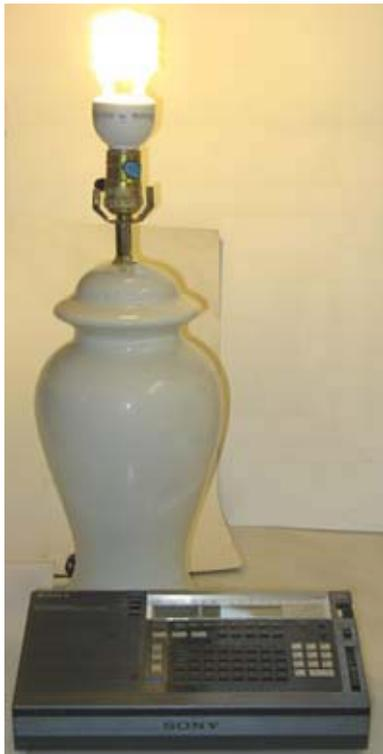
Testing compact fluorescent lamps for RF interference on low, medium and high frequencies. This GE 'Energy Smart' lamp had no RFI warning on the package, but was just as noisy as some earlier models that did have the warning.
