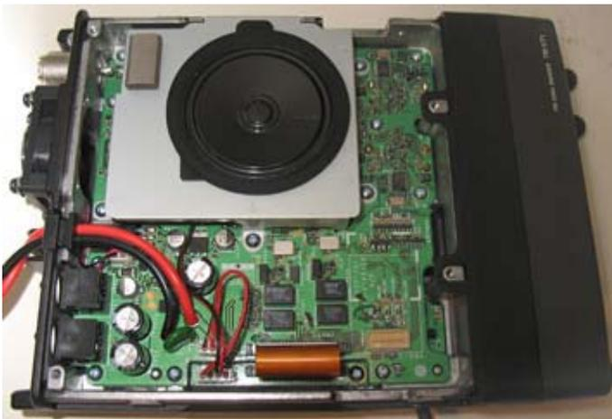
*Inside view of the TM-V71A with top cover removed. At bottom-right, there is an empty connector and space to install the optional VGS-1 Voice Guide and Storage unit.*
