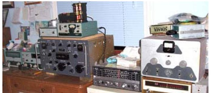
*Karl, N2KZ's shack showing Heath DX-20 crystal-controlled CW transmitter, far right. [See PCARA Update, Oct 2006.]*
