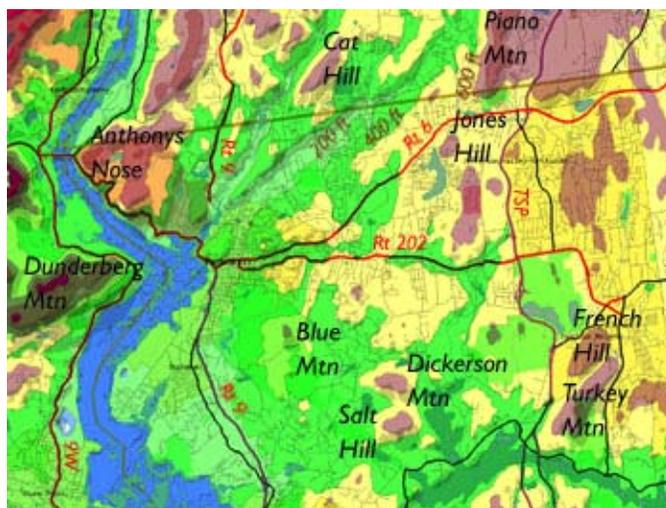
Contour map of Peekskill/Cortlandt area produced by Radio Mobile software, with 200 foot (61 meter) interval. Light green 0-200 ft, dark green 200-400 ft, yellow 400-600 ft, light brown 600-800 ft, mid-brown 800-1000 ft, dark brown over 1000ft.
