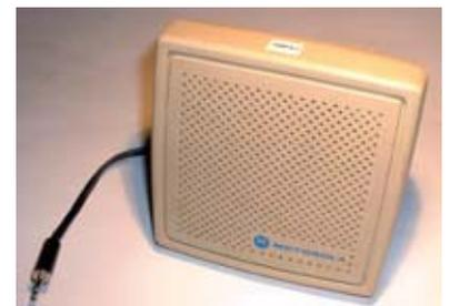
Motorola model contains a large, heavy loudspeaker for mobile use.
