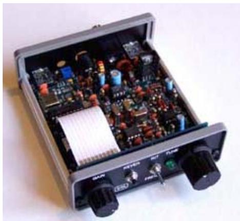
*Small Wonder Labs' DSW-II QRP single band CW transceiver for 7 or 14 MHz*
